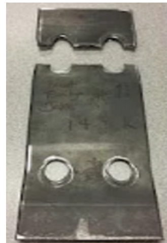
FIGURE 6.11 – Rupture en traction nette
