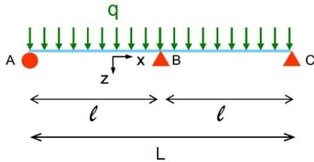
$$q = 40 \text{ KN/m} = 4 \cdot 10^4 \text{ N/m} \quad \text{IPE 100} \quad I_{\text{fort}} = 1,5919 \cdot 10^{-7} \text{ m}^4$$
